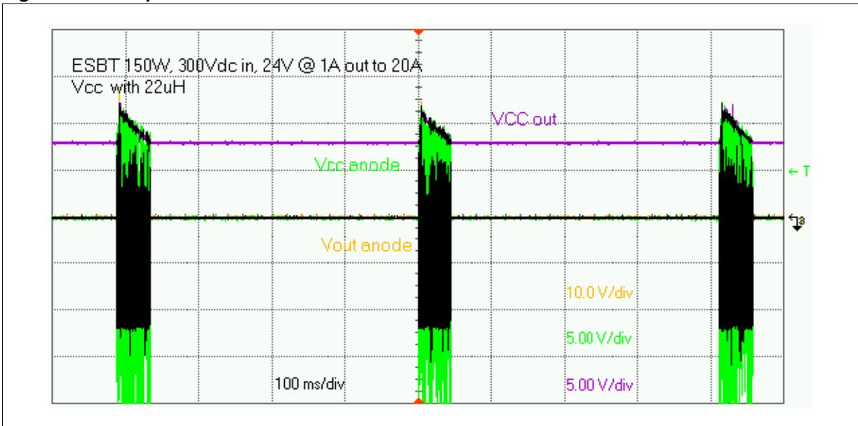
Figure 26. Steady State Vin=850V Pout=150W
