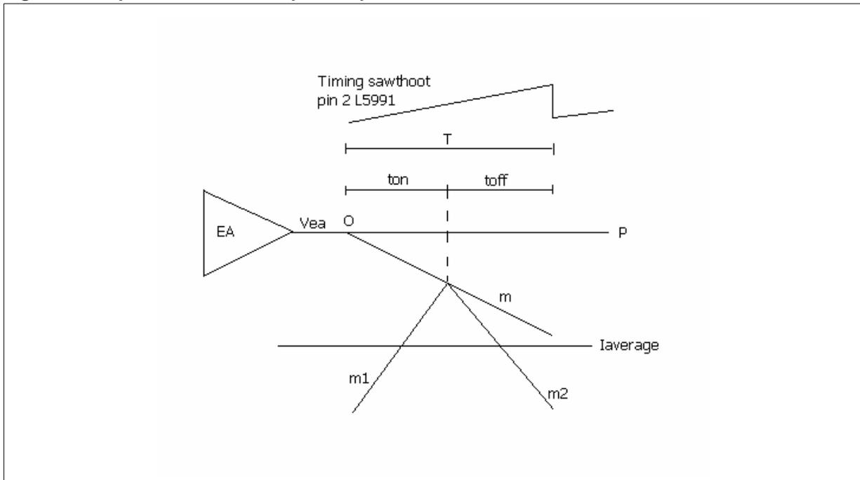
In slope compensation, a negative voltage slope of magnitude  $m=dV_{ea}/dt$  starting at clock time is added to the error amplifier output. The magnitude of  $m$  is, therefore, calculated.
