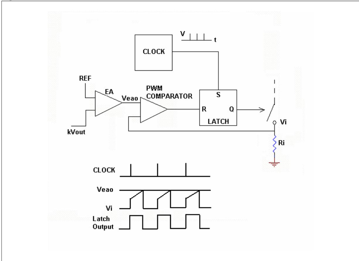
Figure 17. Implementation of Slope Compensation
