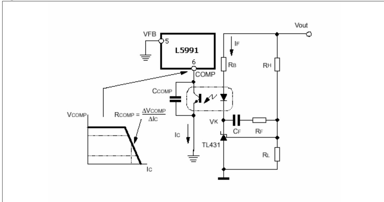
Figure 8. Flyback Frequency Response at Vinmin Adding a Pole at the Origin
