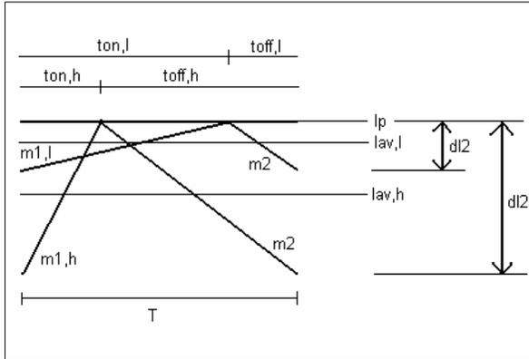
Since the voltage feedback loop keeps the product of  $V_{dcton}$  constant, at lower DC input voltage, where the on time is higher, the average output inductor current  $I_{av}$  is higher, as can be seen from equation 38 and figure 13.
