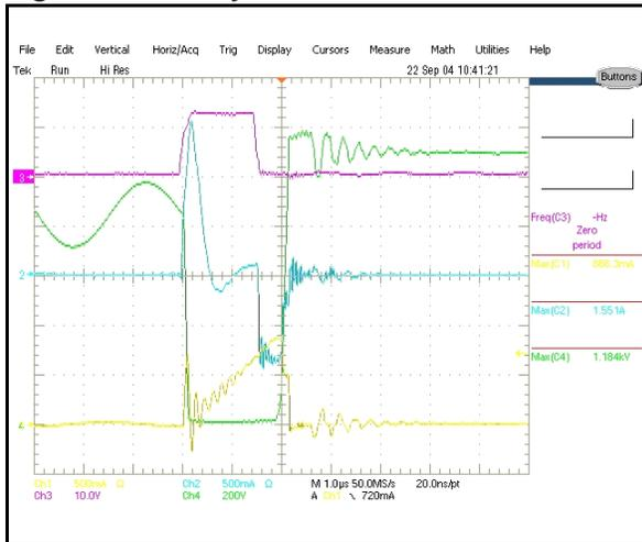
Figure 30, 31, 32 and 33 show the steady state behavior for the low load condition. In this case the switching frequency is about 37KHz, and the collector voltage signal (green waveform) has been added since in this less stressful condition the probe doesn't affect the system stability. From figure 31 is possible to see the very high voltage applied on the collector (1184V) during a normal working condition.
