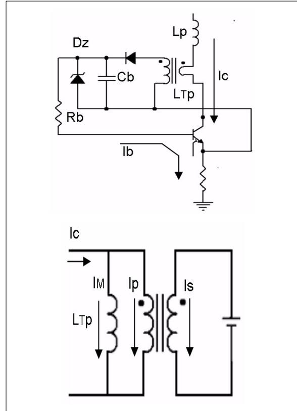
The driving network guarantees a zone with fixed  $I_C/I_B$  ratio that results imposed once the current transformer turn ratio has been chosen. From the ESBT STC08DE150 datasheet, and in particular looking at the storage time characterization, it is clear that a turn ratio equal to 5 is a good value to ensure the right saturation of ESBT at  $I_C = 2A$ , so that in the current transformer we can fix at first:
