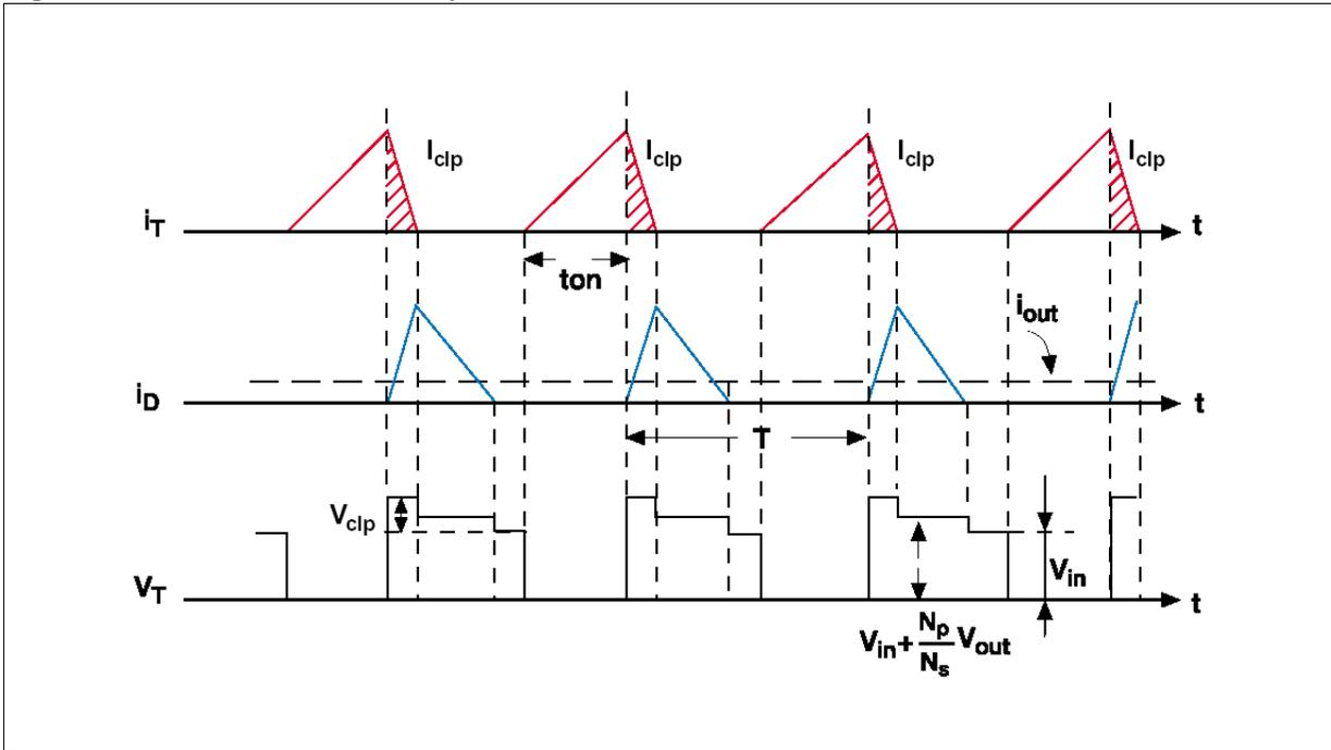
Figure 3. Continuous Mode Flyback Waveforms
