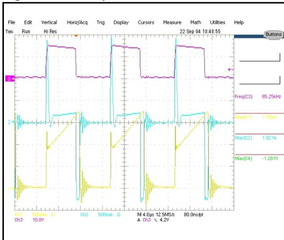
Figure 26, 27, 28, and 29 show the prototype steady state behavior, by reporting the gate voltage (violet waveform), the base current (blue waveform), and the collector current (yellow waveform) signals. The collector voltage signal has been not caught under maximum load condition because the probe parasitic capacitance generates an inner loop noise causing some undesirable oscillations.
