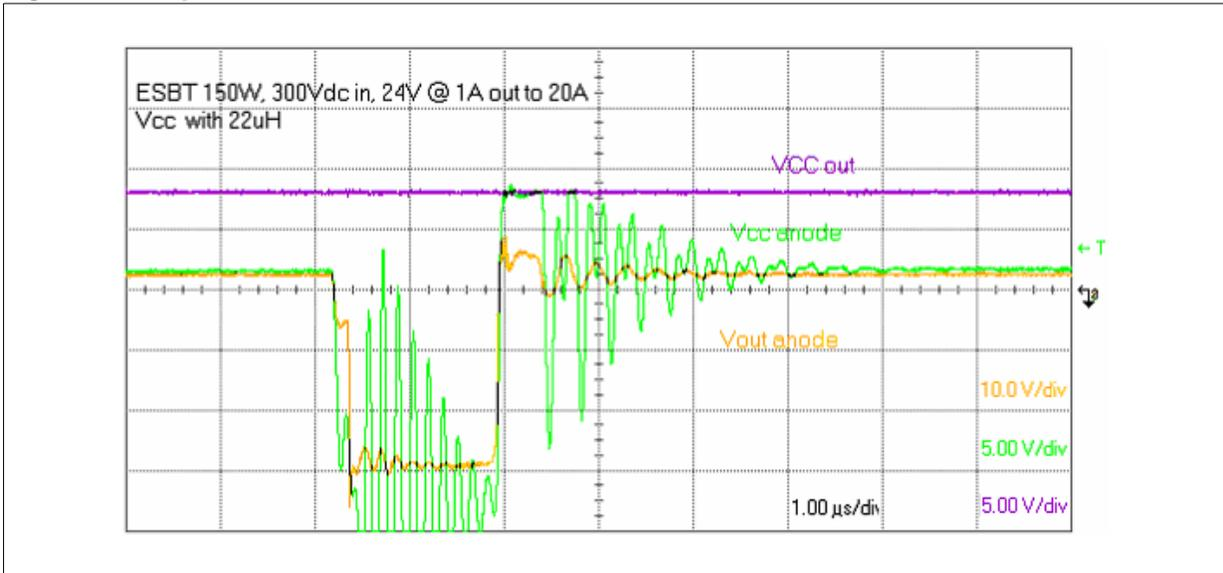
Figure 25. Hiccup Mode with Short Circuit Protection
