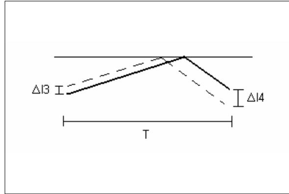
Furthermore, if the duty cycle is less than 50% ( $m_2 < m_1$ ) as in figure 14, the output disturbance  $\Delta I_2$  will be less than the input disturbance  $\Delta I_1$ , and after some cycles, the disturbance will die out. But if the duty cycle is greater than 50% ( $m_2 > m_1$ ) as in figure 15, the output disturbance after one cycle is greater than the input disturbance.
