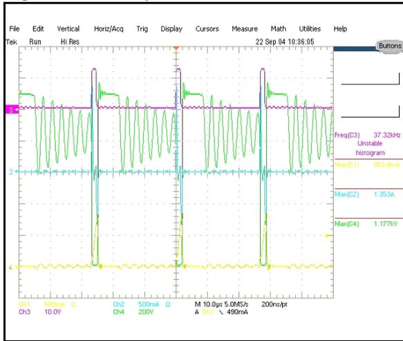
Figure 33. Steady State Vin=250V Pout=25W
