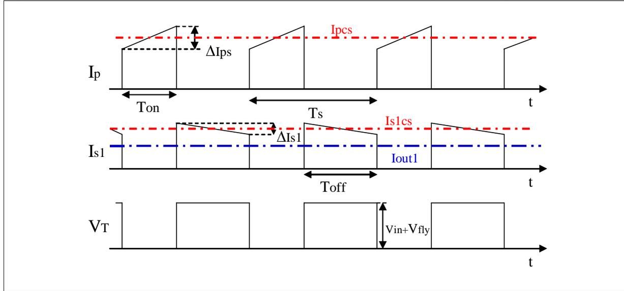
Figure 4 reports the most significant waveforms and relevant nomenclature to further proceed in the flyback design. From figure 4, we define  $I_{PCS}$  the primary average current value and  $\Delta I_{PS}$  the primary current variation during the on time,  $I_{S1CS}$  the secondary average current value and  $\Delta I_{S1}$  the secondary current variation during the off time and  $I_{Out1}$  the secondary average current.
