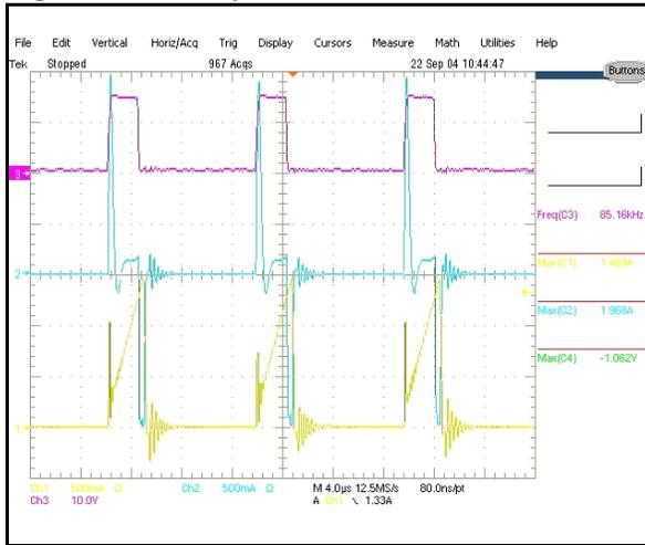
Figure 29. Steady State Vin=250V Pout=150W
